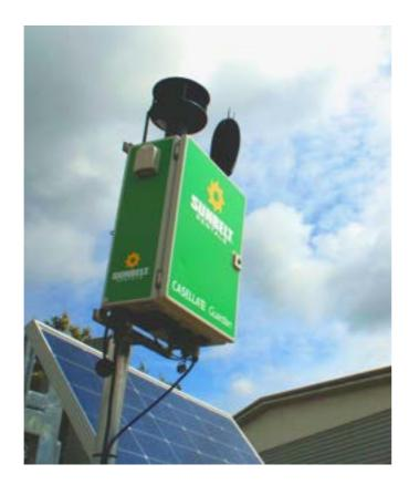
in realtime, should any preset levels be exceeded. Guardians can be powered by a 110 – 240Vac, 12Vdc battery, a combination of both (for generator-powered sites) or a stand-alone solar option. The Guardian can be configured according to your projects needs, and we only charge for the sensors you require.
